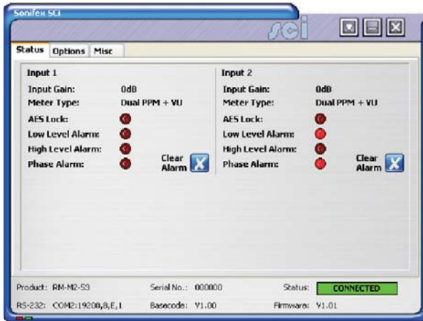
Fig 3-4: Sci Main Status Screen for RM-M2-53
