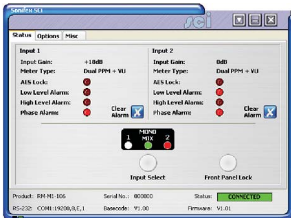
Fig 3-5: SCI Main Status Screen for RM-M1-106
